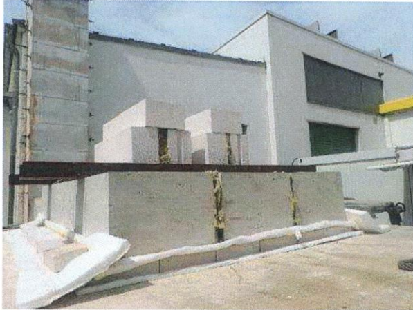
Photo A3-14 View of the side facing away from the fire directly after the fire test
