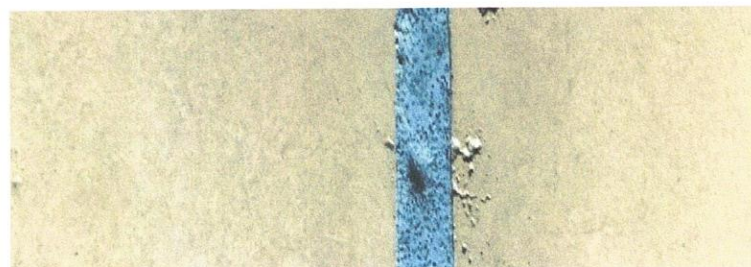
Distance 100 cm, point jet - dirt milling machine - 10 seconds, pressure 100 bar
